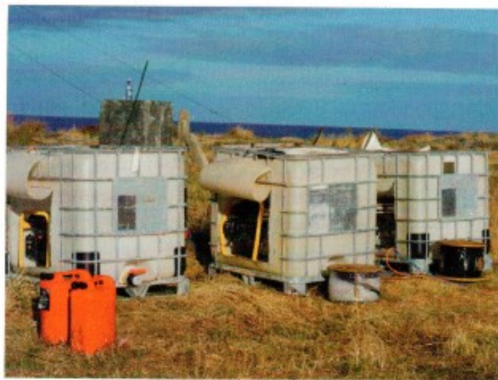
The generators were placed inside depleted fuel containers to mitigate any fuel/oil spills.
