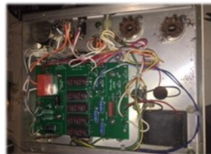
Figure 9 New board wired in and wires dressed
