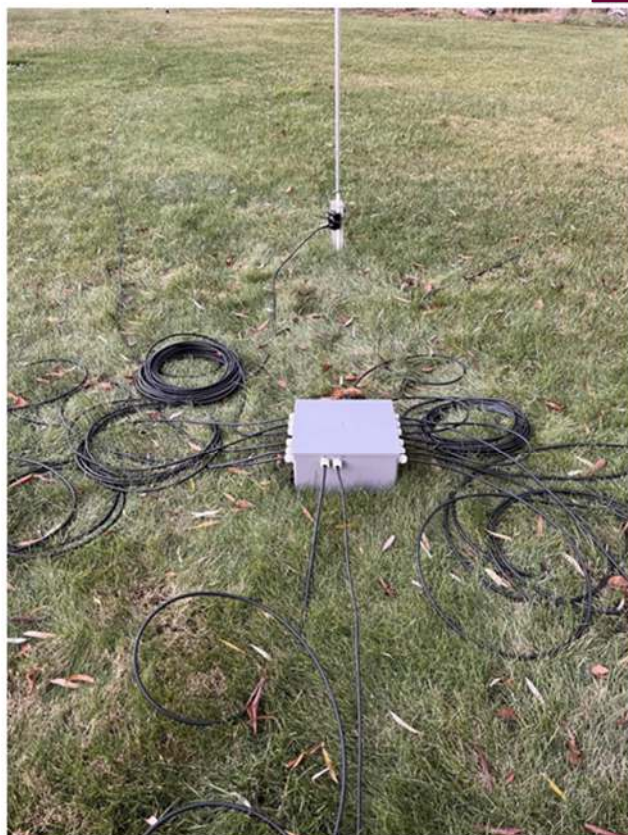
Figure 3. Combiner deployed, coax and center element.
