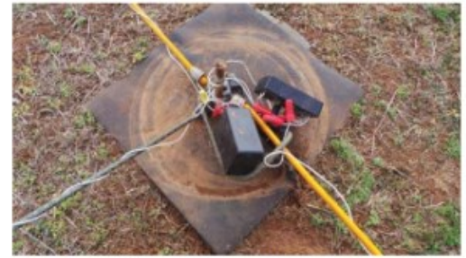
This shows the feedpoint for three Beverages at a single point, each one selected using a remote controlled relay.
