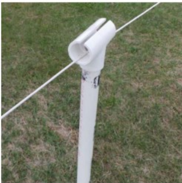
This shows the detail for the top “T” with the slot for the Beverage wire.
