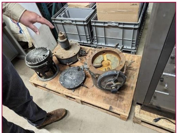
Bill points to a somewhat rusted-out vessel that at one time provided the arc core of an arc transmitter.
