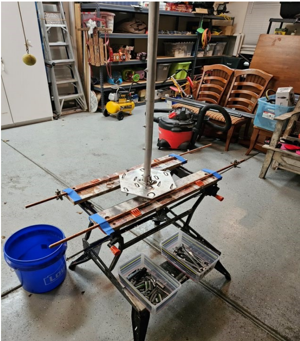
Figure 7 Mast plate and feed point in place - ready for the spreaders.
