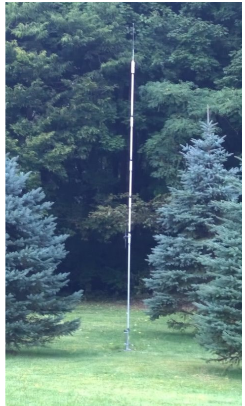
Figure 1 My 6BTV Vertical with the 17M kit installed.
