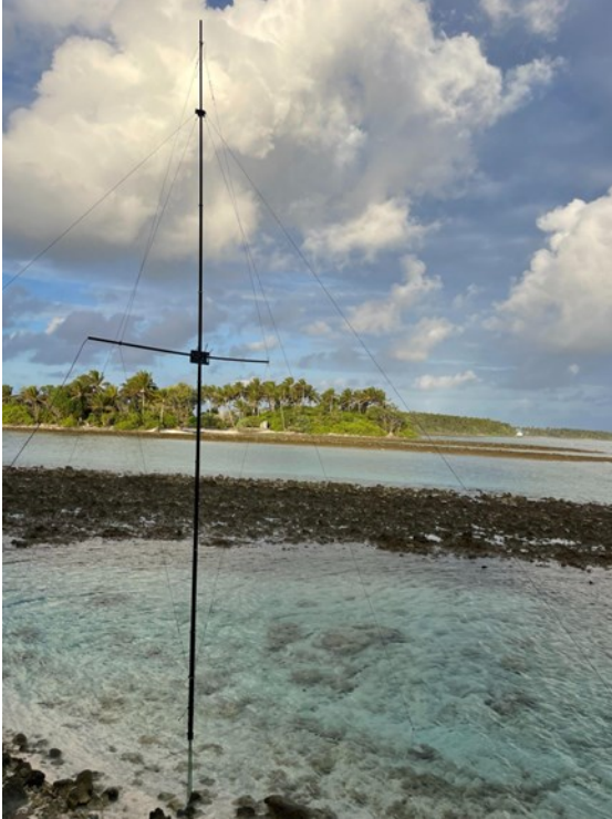
2ele VDA antenna for 15m Band placed within the ocean on Majuro Atoll.
